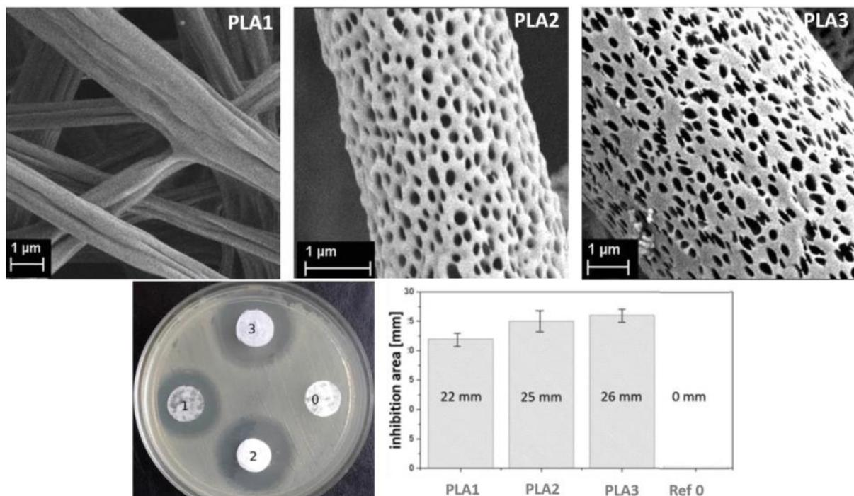
Fig. 1 PLA fibers with different morphologies and the inhibition zone for bacteria of membrane with gentamicine.
